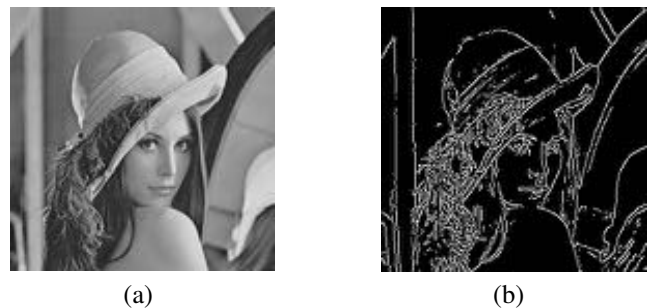
Fig. 1: Edge detection by Canny method (a) A original image (b) A edge detection image.
