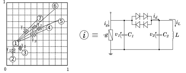
Fig. 3. Coupling between the first chaotic circuit and others.
