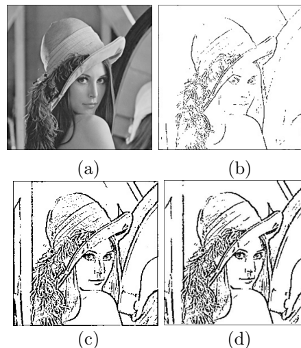
図 2 Simulation results. (a) Input image. (b) Simulation result using the 3 \times 3 template. (c) Simulation result using the 5 \times 5 template. (d) Simulation result of the proposed method ( a = 0.7 ).
