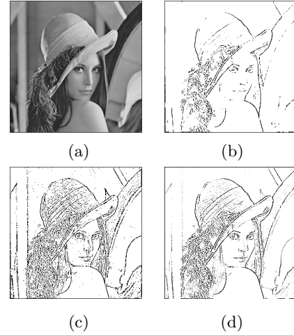
Figure 2: Simulation results of LENA 256x256. (a) Input image. (b) Simulation result of the conventional CNN. (c) Simulation result of the DCNN ( \tau = 0.05 ). (d) Simulation result of the proposed method ( \tau_1 = 0.1 and \tau_2 = 4 ).
