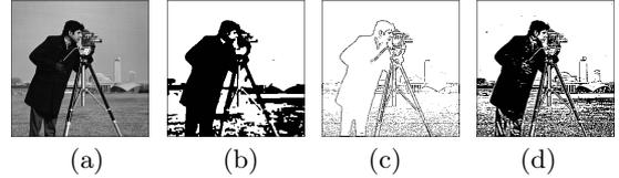
Figure 2: Simulation results. (a) Input image, (b) Binarization by conventional DT-CNN, (c) Edge detection by conventional DT-CNN, (d) First-layer of proposed system.
