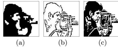
Figure 3: Closeup of simulation results. (a) Binarization by conventional DT-CNN, (b) Edge detection by conventional DT-CNN, (c) First-layer of proposed system.
