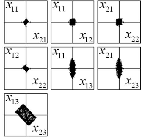
Fig. 3. Phase differences of six resonators.  $\alpha_{C1} = 0.5$ ,  $\alpha_{L1} = 0.3$ ,  $\alpha_{C2} = 0.4$ ,  $\alpha_{L2} = 0.2$ ,  $\gamma = 0.01$ ,  $\varepsilon = 0.055$  and  $\beta = 3.14$ .
