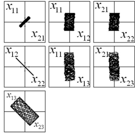
Fig. 6. Phase differences of six resonators.  $\alpha_{C1} = 0.5$ ,  $\alpha_{L1} = 0.3$ ,  $\alpha_{C2} = 0.4$ ,  $\alpha_{L2} = 0.2$ ,  $\gamma = 0.1$ ,  $\varepsilon = 0.055$  and  $\beta = 3.14$ .
