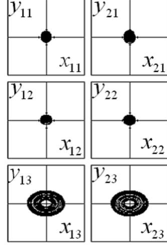
Fig. 2. Lissajous figures of six resonators. Horizontal:  $x_{mn}$ . Vertical:  $y_{mn}$ .  $\alpha_{C1} = 0.5$ ,  $\alpha_{L1} = 0.3$ ,  $\alpha_{C2} = 0.4$ ,  $\alpha_{L2} = 0.2$ ,  $\gamma = 0.01$ ,  $\varepsilon = 0.055$  and  $\beta = 3.14$ .
