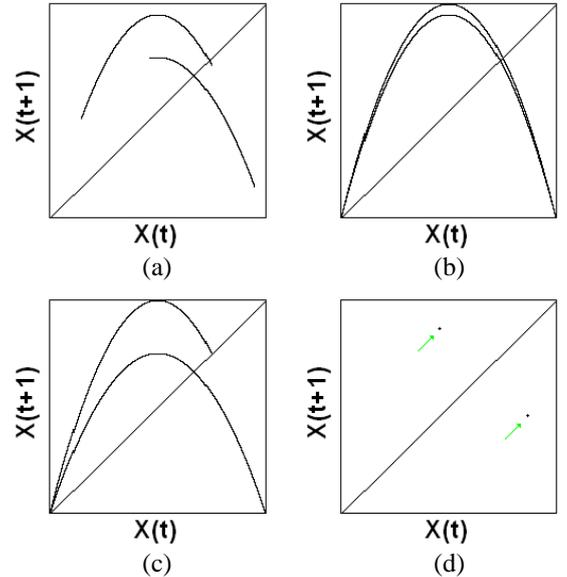
Fig. 2. Return maps of parametrically forced logistic maps for  $\tau = 1$ . (a)  $\alpha_1 = 3.0$  and  $\alpha_2 = 3.8$ . (b)  $\alpha_1 = 3.8$  and  $\alpha_2 = 4.0$ . (c)  $\alpha_1 = 3.0$  and  $\alpha_2 = 4.0$ . (d)  $\alpha_1 = 3.5$  and  $\alpha_2 = 4.0$ .
