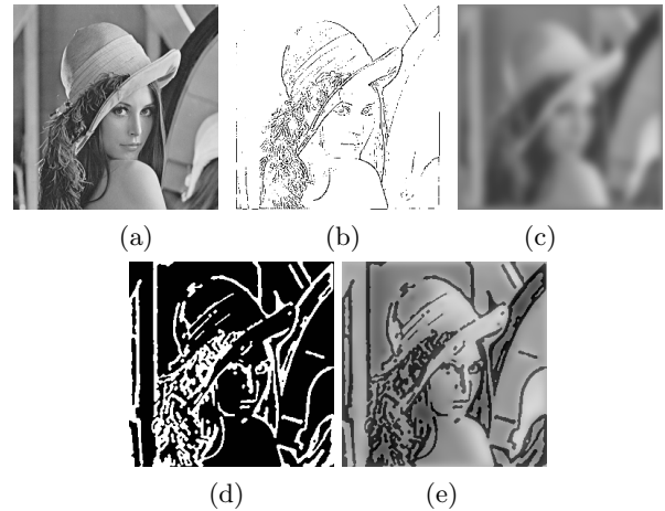
Figure 1: Simulation results. (a) Input image. (b) Edge detection result using the CNN. (c) Diffusion result using template (4). (d) Output image of second layer in our two-layer CNN. (e) Output image of first layer in our two-layer CNN.
