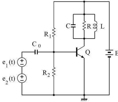
Fig. 1 Base modulation circuit.
