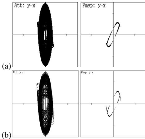
Fig. 4. Examples of chaotic attractors and Poincaré maps observed from each subcircuit,  $\alpha = 0.95$  and  $\omega = 1.50$ . (a)  $\varepsilon = 1.0$ . (b)  $\varepsilon = 1.5$ .
