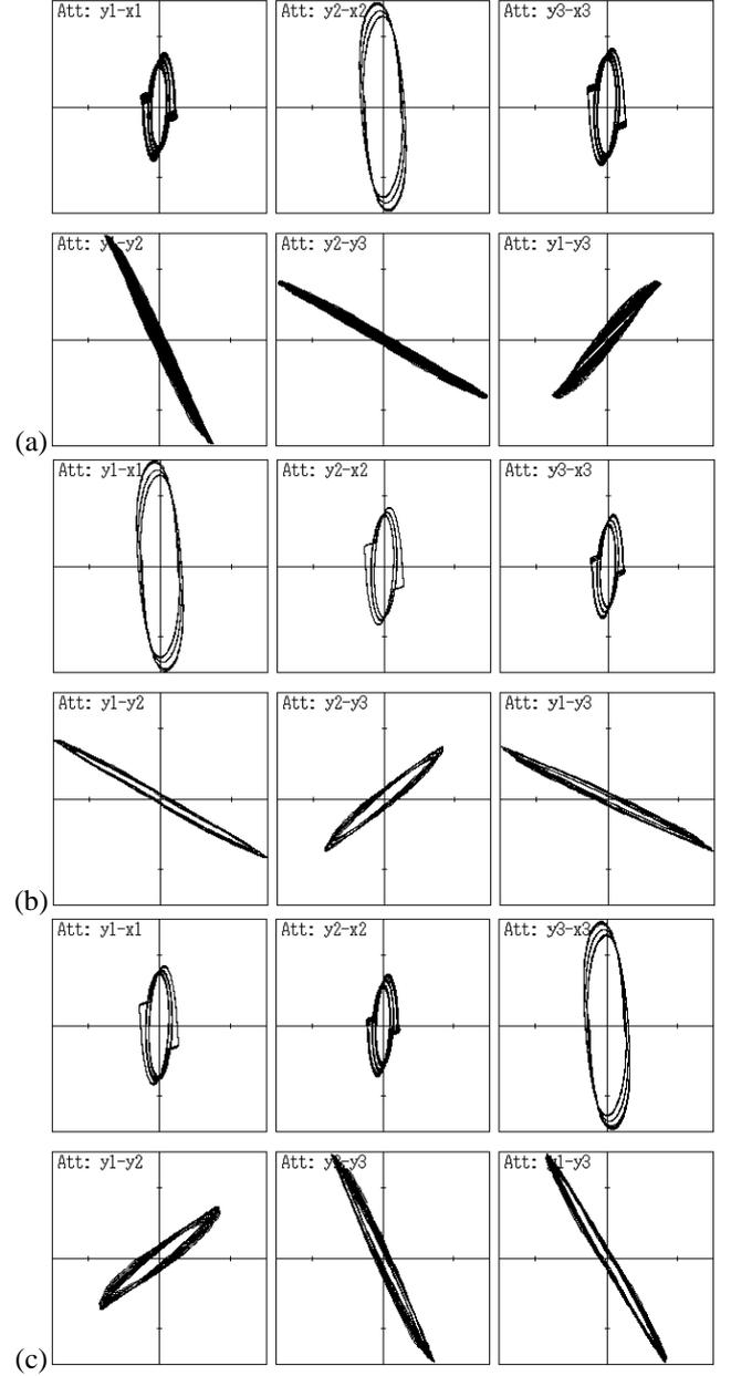
Fig. 7. Attractors and phase differences.  $\varepsilon = 1.50$ ,  $\alpha = 0.95$ ,  $\omega = 1.50$  and  $\delta = 0.80$ .
