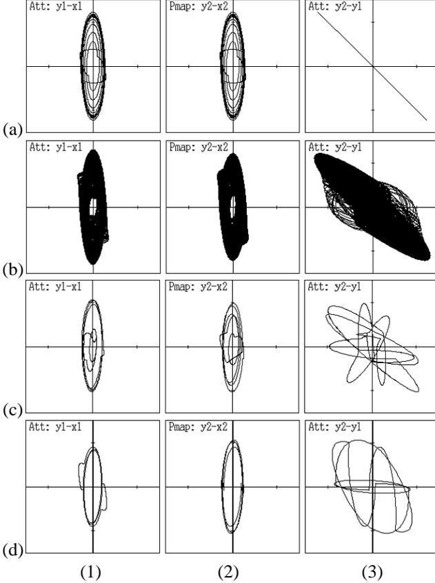
Fig. 6. Attractors and phase differences.  $\varepsilon = 1.35$ ,  $\alpha = 0.95$ ,  $\omega = 1.50$  and  $\delta = 0.80$ . Phase difference of rectangular wave: (a) 0, (b)  $\pi/20$ , (c)  $\pi/4$  and (d)  $\pi$ . (1)  $x_1$  versus  $y_1$ . (2)  $x_2$  versus  $y_2$ . (3)  $y_1$  versus  $y_2$ .
