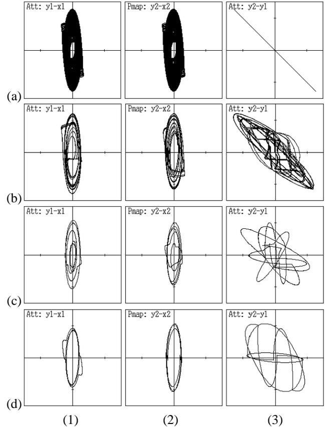
Fig. 5. Attractors and phase differences.  $\varepsilon = 1.50$ ,  $\alpha = 0.95$ ,  $\omega = 1.50$  and  $\delta = 0.80$ . Phase difference of rectangular wave: (a) 0, (b)  $\pi/20$ , (c)  $\pi/4$  and (d)  $\pi$ . (1)  $x_1$  versus  $y_1$ . (2)  $x_2$  versus  $y_2$ . (3)  $y_1$  versus  $y_2$ .
