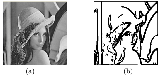
Figure 2: Simulation results of edge detection using the proposed SWCNN system. (a) Input image. (b) Output image using the proposed SWCNN system.
