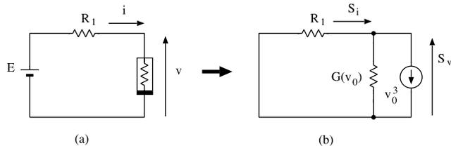
**Fig. 3** (a) Simple nonlinear resistive circuit, (b) the sensitivity circuit for the optimization parameter  $c_3$ .
