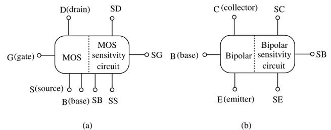
**Fig. A. 2** MOSFET and bipolar transistor sensitivity modules.
