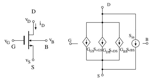
**Fig. 7** (a) nMOS, (b) nMOS sensitivity module.
