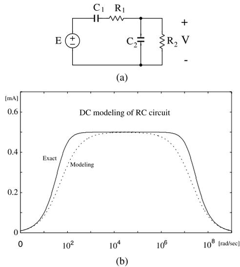
**Fig. 9** (a) A simple RC circuit. (b) Frequency response curves.  $R_1 = R_2 = 10$  [k $\Omega$ ],  $C_1 = 1$  [ $\mu$ F],  $C_2 = 10$  [pF].
