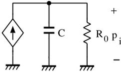
**Fig. 5** A circuit configuration for attaining the maximum gain under low power consumption and the slew-rate.
