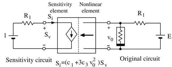
**Fig. A. 1** Coupling of the original and the sensitivity circuits.
