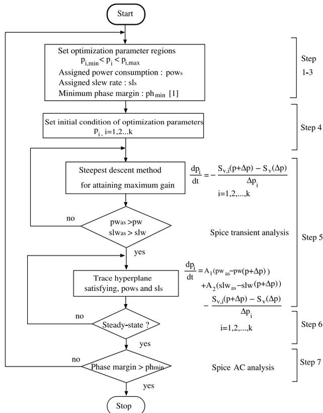
**Fig. 6** Flowchart of our steepest descent algorithm based on the nonlinear programming.
