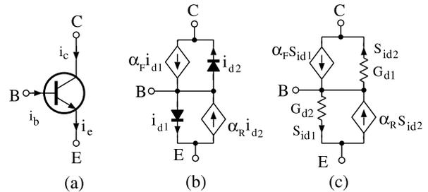
Fig. 8 (a) NPN bipolar transistor, (b) Ebers-Moll model, (c) sensitivity module of transistor.
