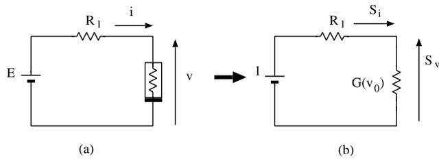
**Fig. 2** (a) Simple nonlinear resistive circuit, (b) the sensitivity circuit to optimization parameter  $E$ .
