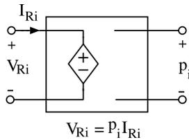
Fig. A-3 Resistance transformation circuit.
