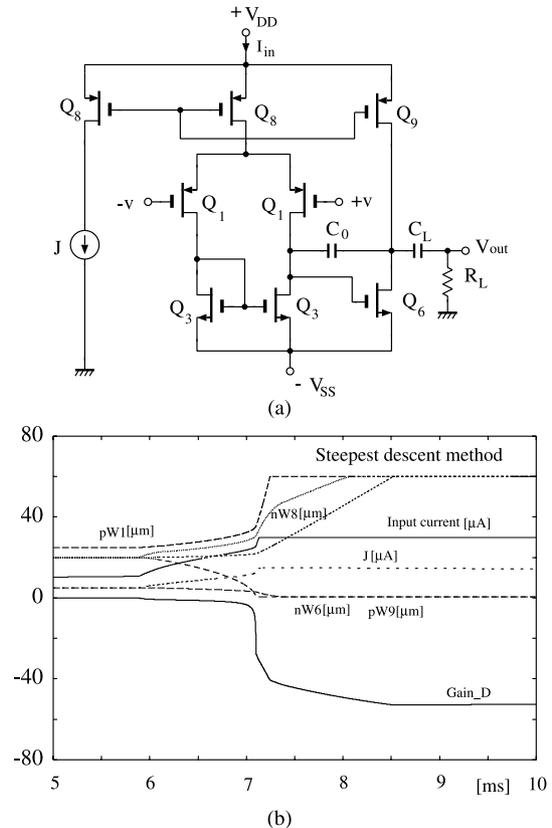
**Fig. 10** (a) Two stage CMOS amplifier. (b) Optimization of two-stage CMOS amplifier.  $V_{DD} = 2.5$  [V],  $V_{SS} = -2.5$  [V], Frequency = 100 [MHz],  $C_0 = 0.1$  [nF],  $C_L = 1$  [nF],  $R_L = 1000$  [k $\Omega$ ].
