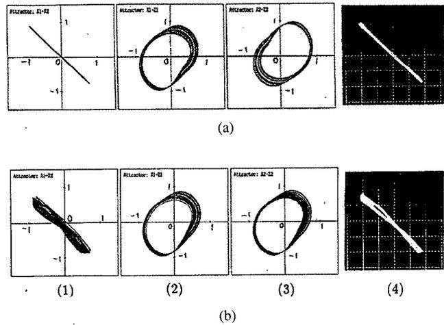
Fig. 3. Synchronization of two asymmetric chaos.  $\gamma = 0.10$  ( $R = 190 \Omega$ ). (a) Symmetric synchronization for  $\beta = 0.287$  ( $r = 554 \Omega$ ). (b) Asymmetric synchronization for  $\beta = 0.308$  ( $r = 586 \Omega$ ). (1)  $x_1$  versus  $x_2$ . (2)  $x_1$  versus  $z_1$ . (3)  $x_2$  versus  $z_2$ . (4) Circuit experimental results.  $I_1$  versus  $I_2$ . 0.4 mA/div.
