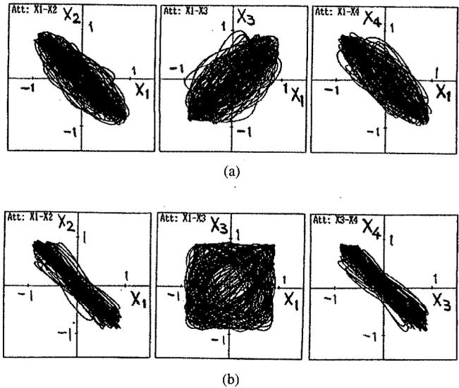
Fig. 6. Quasi-synchronization of four symmetric chaos (computer calculated results).  $\beta = 0.30$ . (a) In and opposite-phases quasi-synchronization for  $\gamma = 0.40$ . (b) Two pairs of opposite-phase quasi-synchronizations for and  $\gamma = 0.10$ .
