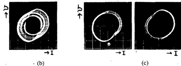
Fig. 1. Circuit model. (a) Chaotic circuits coupled by one resistor. (b) Symmetric chaotic attractor ( $r = 650 \Omega$ ). (c) Coexistence of two asymmetric chaotic attractors ( $r = 554 \Omega$ ). Horizontal: 0.4 mA/div. Vertical: 1 V/div.
