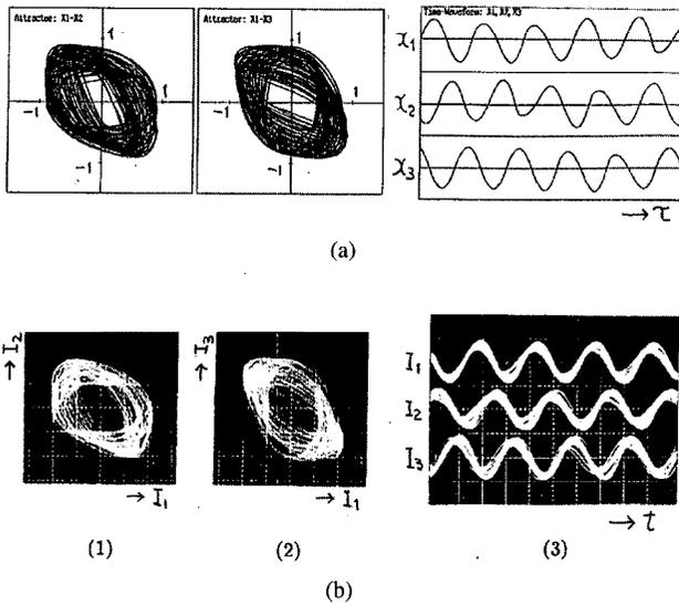
Fig. 4. Three-phase quasi-synchronization of three symmetric chaos. (a) Computer calculated results.  $\beta = 0.305$  and  $\gamma = 0.05$ . (a1)  $x_1$  versus  $x_2$ . (a2)  $x_1$  versus  $x_3$ . (a3) Time-waveforms. (b) Circuit experimental results.  $r = 650 \Omega$  and  $R = 50.8 \Omega$ . (b1)(b2) 0.4 mA/div. (b3) Horizontal: 0.2 ms/div. Vertical: 1 mA/div.
