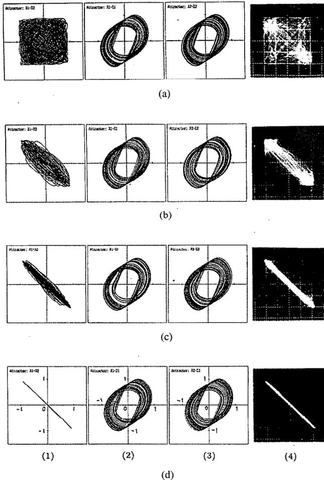
Fig. 2. Synchronization of two symmetric chaos.  $\beta = 0.325$  ( $r = 650 \Omega$ ). (a)  $\gamma = 0.0$  ( $R = 0 \Omega$ ). (b)  $\gamma = 0.10$  ( $R = 48 \Omega$ ). (c)  $\gamma = 0.22$  ( $R = 292 \Omega$ ). (d)  $\gamma = 0.35$  ( $R = 540 \Omega$ ). (1)  $x_1$  versus  $x_2$ . (2)  $x_1$  versus  $z_1$ . (3)  $x_2$  versus  $z_2$ . (4) Circuit experimental results.  $I_1$  versus  $I_2$ . 0.4 mA/div.
