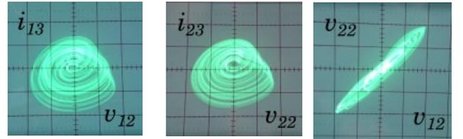
Figure 3: Attractors and synchronization phenomena in the circuit experiment.
