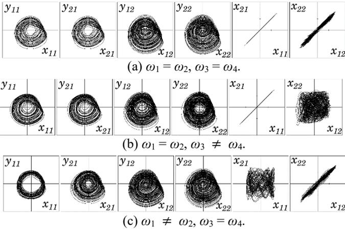
Figure 2: Attractors and synchronization phenomena in the computer simulation.
