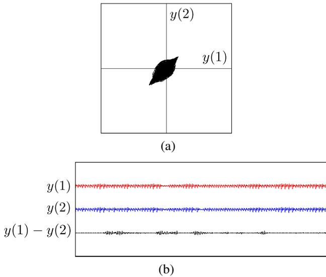
Figure 3: Simulation result.  $\delta = 0.2$ ,  $a = 0.2$ ,  $b = 10.0$ . (a)Lissajous figure. (b)Waveform.
