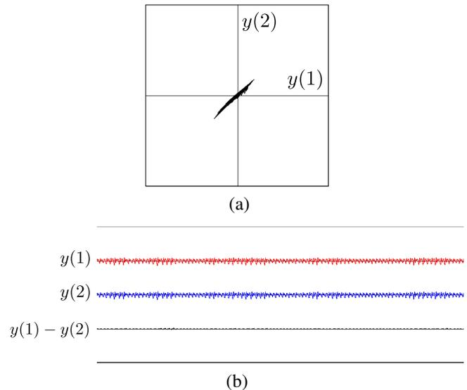
Figure 4: Simulation result.  $\delta = 0.6$ ,  $a = 0.2$ ,  $b = 10.0$ . (a)Lissajous figure. (b)Waveform.
