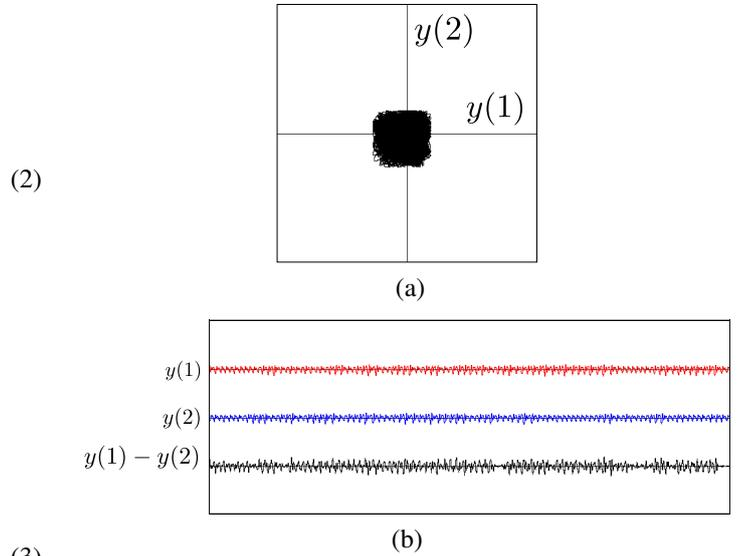
Figure 2: Simulation result.  $\delta = 0.0000001$ ,  $a = 0.2$ ,  $b = 10.0$ . (a)Lissajous figure. (b)Waveform.
