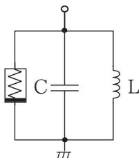
Figure 1: van del pol oscillator.
