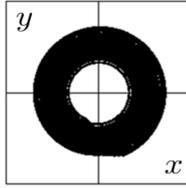
Figure 3: Chaotic attractor obtained by computer simulation.
