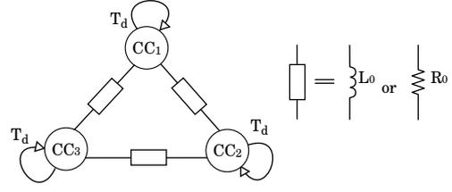
Figure 4: Ring coupled system by resistors.
