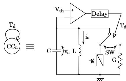
Figure 1: Time delayed chaotic circuit.
