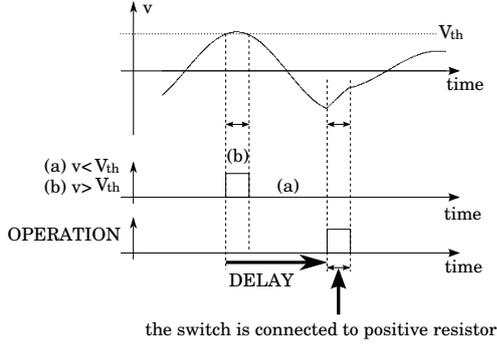
Figure 2: Switching operation.
