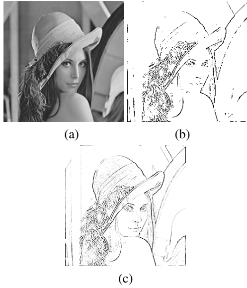
Figure 5: Simulation results. (a) Input image. (b) Simulation result of the conventional CNN. (c) Simulation result of the proposed method ( T_\alpha = 1 , -0.2 \leq \alpha \leq 0 , T_\beta = 5 , 0 \leq \beta \leq 0.1 ).
