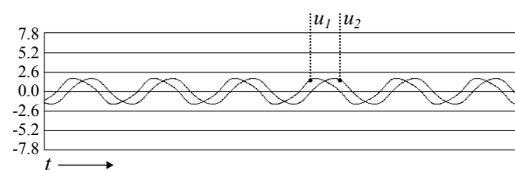
Figure 2: Oscillation of the general neural oscillator ( $W_{positive} = 2.0$ ,  $W_{negative} = -2.0$ ,  $\tau = 2.0$ ).
