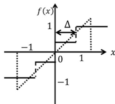
Fig. 2. The output characteristic of DT-CNN.
