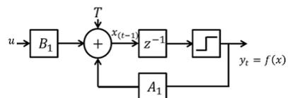
Fig. 1. Block diagram of the DT-CNN.
