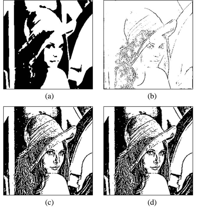
Fig. 6. Simulation results of binarization 1. (a) Simulation result of binarization by using conventional DT-CNN, (b) Simulation result of edge detection by using conventional DT-CNN, (c) Simulation result for first-layer of proposed system. (d) Simulation result for first-layer of proposed system.
