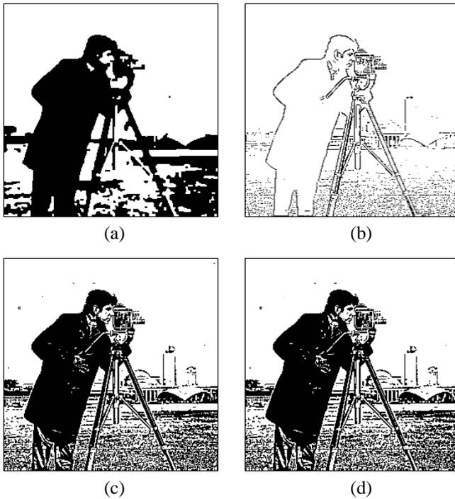
Fig. 8. Simulation results of binarization 2. (a) Simulation result of binarization by using conventional DT-CNN, (b) Simulation result of edge detection by using conventional DT-CNN, (c) Simulation result for first-layer of proposed system. (d) Simulation result for first-layer of proposed system.
