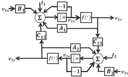
Fig. 3. Block diagram of the two-layer CNN.
