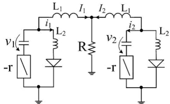
Fig. 1. Two coupled chaotic circuits model [1].
