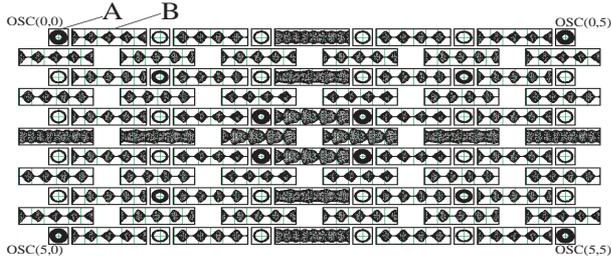
Figure 2: Computer simulation result of the phase-inversion waves in in-and-anti-phase synchronization when  $N = 6$ .
