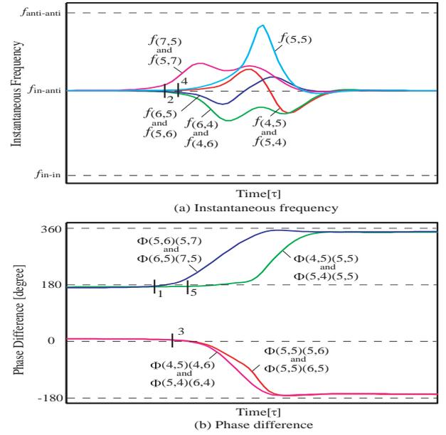
Figure 5: Transitions of phase difference and frequencies by penetration between two phase-inversion waves on in-and-anti-phase synchronization.
