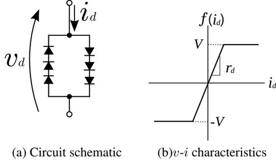
Figure 3: Coupled diodes model
