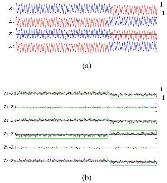
Figure 9: Anti-phase synchronization of switching phenomena in the case of  $N = 4$ .  $\alpha = 0.40$ ,  $\beta = 3.0$ ,  $\gamma = 470.0$  and  $\delta = 0.095$ .
