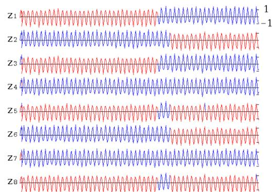
Figure 10: Anti-phase synchronization of switching phenomena in the case of  $N = 8$ .  $\alpha = 0.40$ ,  $\beta = 3.0$ ,  $\gamma = 470.0$  and  $\delta = 0.043$ .
