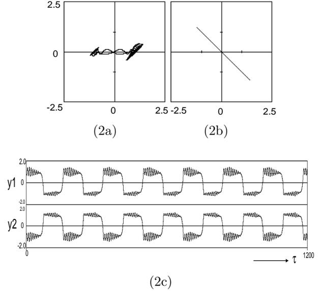
Figure 3: State transition phenomenon around anti-phase synchronization (computer calculated result).  $\alpha = 2.0$ ,  $\beta = 4.0$ ,  $\gamma = 0.1$ , and  $\delta = 0.0014$ . (1) Cross-coupled chaotic circuits. (2) Direct-coupled chaotic circuits. (a) Attractor on  $y_1 - z_1$  plane. (b) Attractor on  $y_1 - y_2$  plane. (c) Time waveform.
