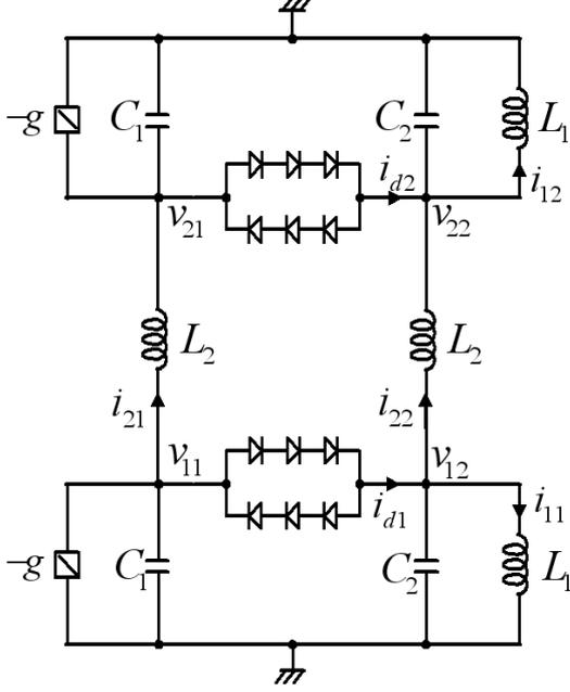
Figure 2: Direct-coupled chaotic circuits.
