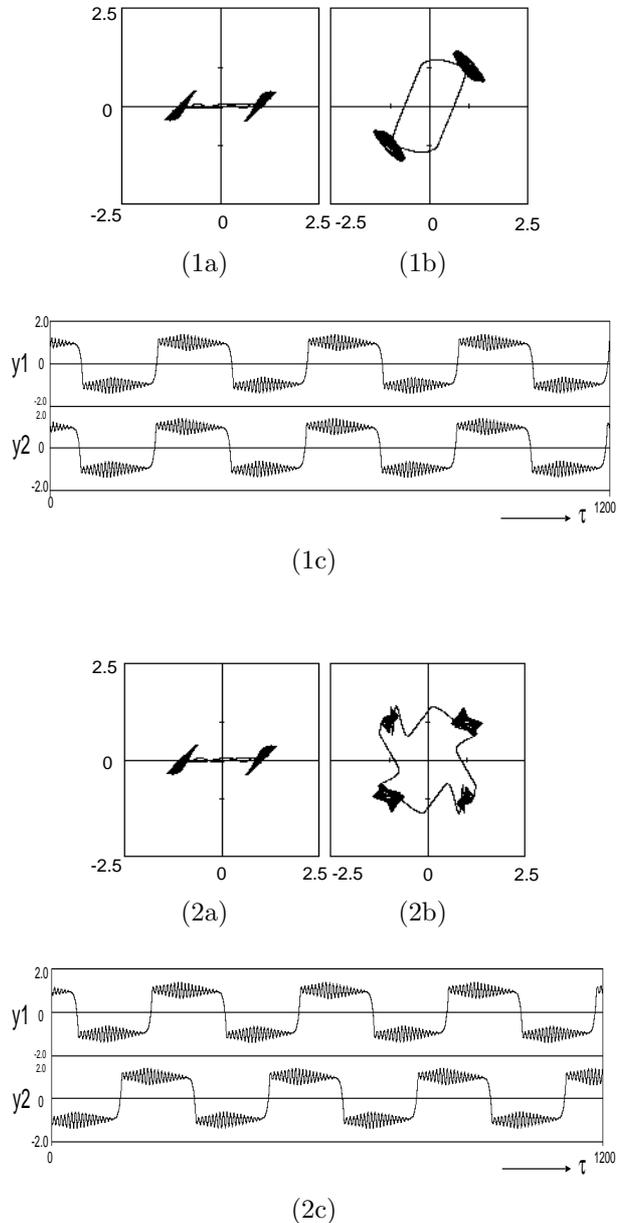
Figure 4: State transition phenomenon observed from cross-coupled chaotic circuits (computer calculated result).  $\alpha = 2.0$ ,  $\beta = 4.0$ ,  $\gamma = 0.1$ , and  $\delta = 0.0014$ . (1) Around in-phase synchronization. (2) Around quadrature-phase synchronization. (a) Attractor on  $y_1 - z_1$  plane. (b) Attractor on  $y_1 - y_2$  plane. (c) Time waveform.
