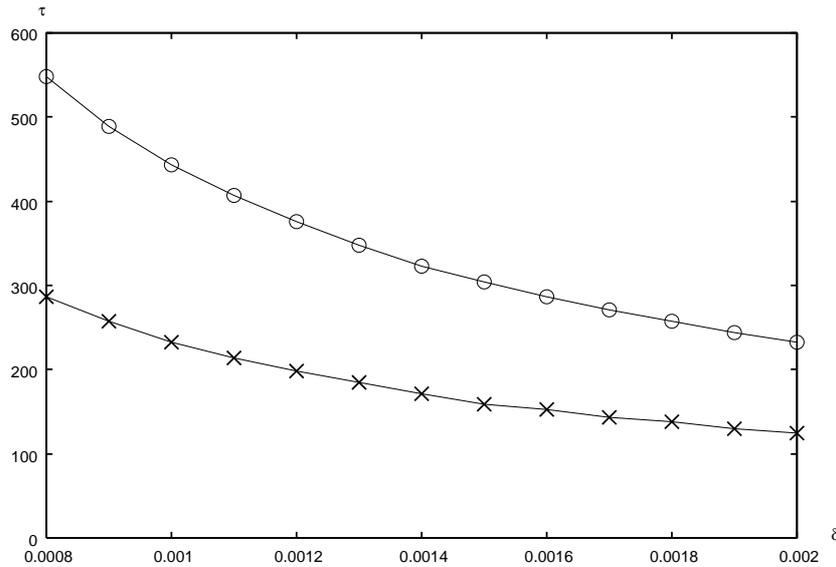
Figure 5: Sojourn time between state transitions versus coupling parameter (anti-phase synchronization).  $\alpha = 2.0$ ,  $\beta = 4.0$ ,  $\gamma = 0.1$ , and  $\delta = 0.0014$ . Circle: Cross-coupled. Cross: Direct-coupled.
