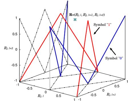
Figure 4: Operation of Our Suboptimal Receiver ( $N_d = 3$ ).
