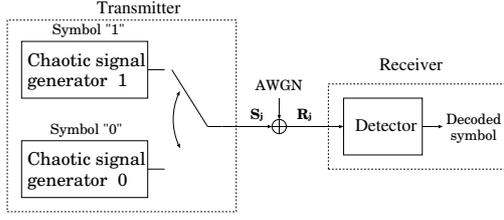
Figure 1: Block diagram of discrete-time binary CSK communication system.
