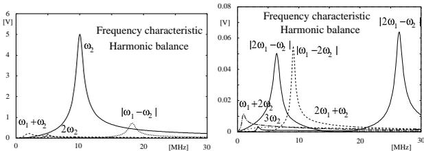
Fig. 9 (a) Frequency characteristic by HB. (b) Other frequency components.
