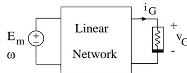
Fig. 1 Nonlinear resistive circuit.
