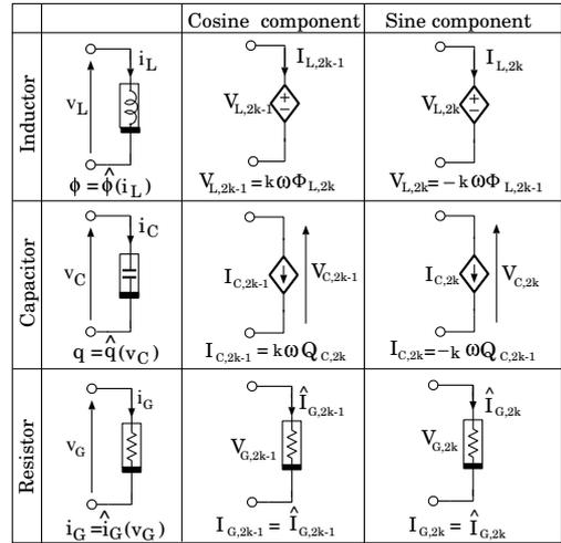
Fig. 3 Sine-Cosine equivalent circuit models.
