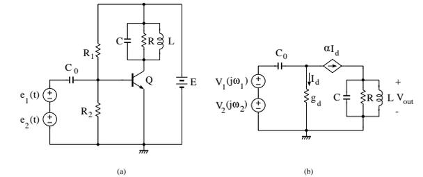
Fig. 7 (a) Base modulation circuit. (b) 1st order Volterra equivalent circuit.
