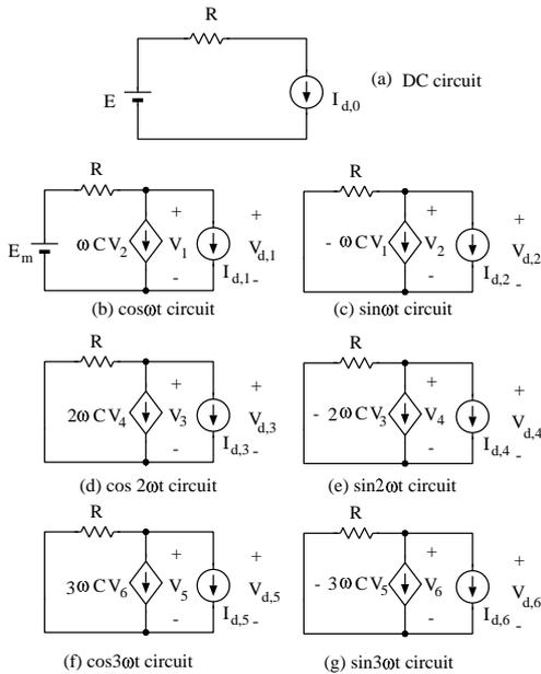
Fig. 5 Equivalent HB circuit of Fig. 4.
