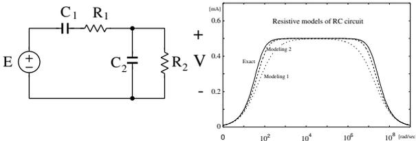
Fig.5(a) A simple RC circuit, (b) Frequency response curves.  $R_1 = R_2 = 10[k\Omega]$ ,  $C_1 = 1[\mu F]$ ,  $C_2 = 10[pF]$
