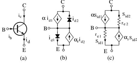
Fig.4(a) NPN bipolar transistor, (b) Ebers-Moll model, (c) sensitivity module of transistor module.
