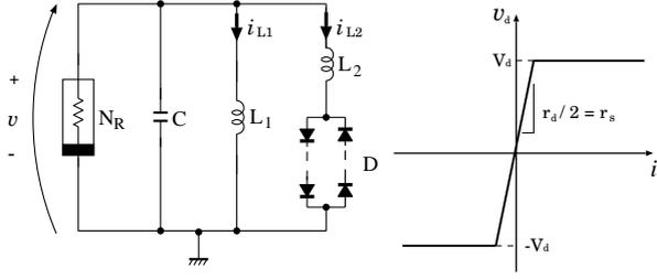
Figure 1: Based chaotic circuit with piecewise linear resistors.
