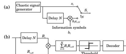
Figure 8: DCSK operation. (a) transmitter. (b) receiver.
