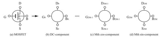
Fig. 2. HB module of the MOSFET.
