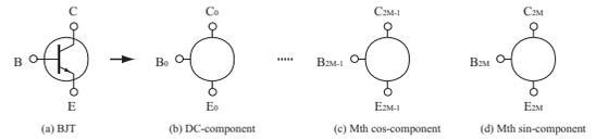
Fig. 1. HB module of the bipolar transistor.
