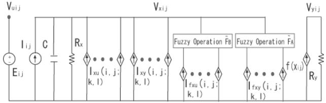
Fig. 1 Circuit of cell  $C_{ij}$  in Fuzzy CNN.
