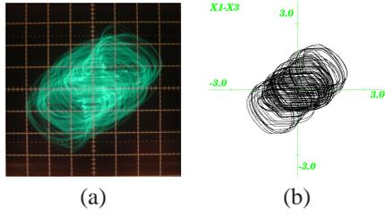
Figure 6: circuit experimental result (a) and computer calculated result (b) of circuit no. 2. (a)horizontal axis:  $v_1$ [0.5v/div], vertical axis: $v_3$ [0.5v/div],  $R_1 = 3.3$ [k $\Omega$ ],  $R_2 = 2.4$ [k $\Omega$ ],  $R_3 = 1.0$ [k $\Omega$ ],  $R_4 = 2.7$ [k $\Omega$ ],  $C_1 = C_2 = C_3 = 33$ [nF],  $L_1 = 50$ [mH]. (b)horizontal axis:  $x_1$ , vertical axis:  $x_3$ ,  $\alpha = 1.2$ ,  $\beta = 2.7$ ,  $\gamma = 1.0$ ,  $\delta = 7$ ,  $\varepsilon = 20$ .
