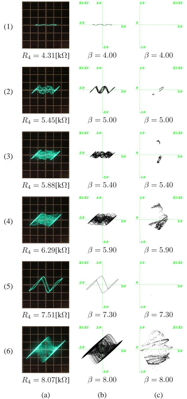
Figure 5: (a)circuit experimental results, (b)computer calculated results, (c) Poincaré maps. (a)horizontal axis:  $v_1$ [0.5v/div], vertical axis:  $v_3$ [0.5v/div],  $R_1 = 2.0$ [k $\Omega$ ],  $R_2 = 5.6$ [k $\Omega$ ],  $R_3 = 1.0$ [k $\Omega$ ],  $C_1 = C_2 = C_3 = 33$ [nF],  $L_1 = 10$ [mH]  $R_4$ . (b)horizontal axis:  $x_1$ , vertical axis:  $x_3$ ,  $\alpha = 0.6$ ,  $\gamma = 1.1$ ,  $\delta = 43$ ,  $\varepsilon = 30$ .
