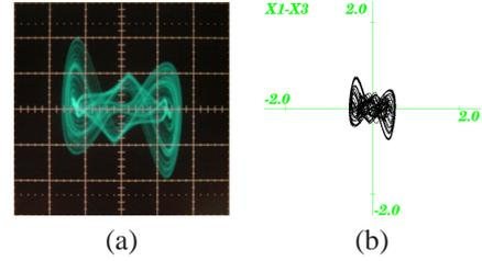
Figure 9: circuit experimental result (a) and computer calculated result (b) of circuit no. 5. (a)horizontal axis:  $v_1$ [0.2v/div], vertical axis: $v_3$ [0.2v/div],  $R_1 = 5.6$ [k $\Omega$ ],  $R_2 = 5.6$ [k $\Omega$ ],  $R_3 = 1.0$ [k $\Omega$ ],  $R_4 = 3.1$ [k $\Omega$ ],  $C_1 = C_2 = C_3 = 33$ [nF],  $L_1 = 50$ [mH]. (b)horizontal axis:  $x_1$ , vertical axis:  $x_3$ ,  $\alpha = 1.0$ ,  $\beta = 3.0$ ,  $\gamma = 1.0$ ,  $\delta = 20$ ,  $\varepsilon = 40$ .
