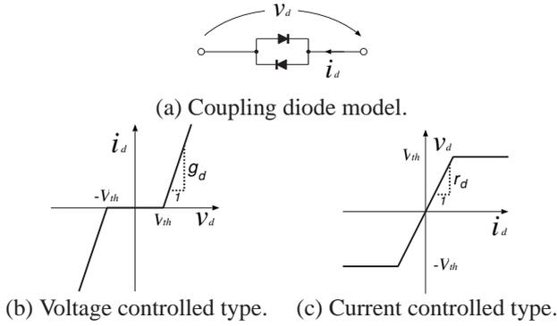
Figure 4: Coupling diode model and its characteristics
