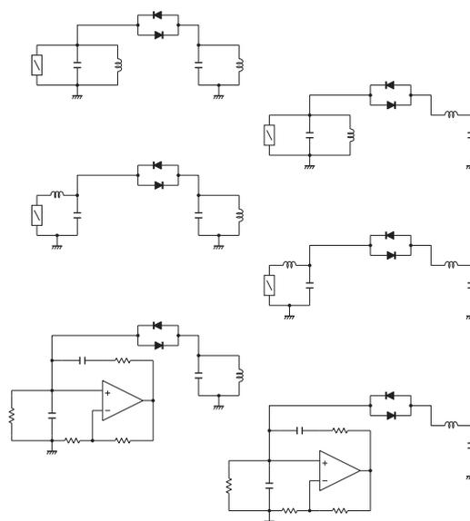
Figure 2: Chaotic circuits developed by our designing method.
