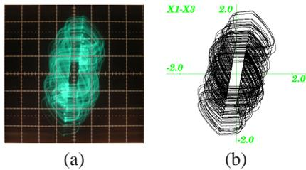
Figure 8: circuit experimental result (a) and computer calculated result (b) of circuit no. 4. (a)horizontal axis:  $v_1$ [0.5v/div], vertical axis: $v_3$ [0.5v/div],  $R_1 = 3.3$ [k $\Omega$ ],  $R_2 = 2.7$ [k $\Omega$ ],  $R_3 = 1.0$ [k $\Omega$ ],  $R_4 = 3.1$ [k $\Omega$ ],  $C_1 = C_2 = C_3 = 33$ [nF],  $L_1 = 50$ [mH]. (b)horizontal axis:  $x_1$ , vertical axis:  $x_3$ ,  $\alpha = 1.6$ ,  $\beta = 2.1$ ,  $\gamma = 1.0$ ,  $\delta = 6$ ,  $\varepsilon = 20$ .
