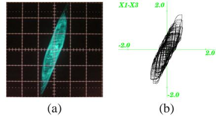
Figure 10: circuit experimental result (a) and computer calculated result (b) of circuit no. 6. (a)horizontal axis:  $v_1$ [0.5v/div], vertical axis: $v_3$ [0.5v/div],  $R_1 = 3.3$ [k $\Omega$ ],  $R_2 = 3.3$ [k $\Omega$ ],  $R_3 = 1.0$ [k $\Omega$ ],  $R_4 = 4.5$ [k $\Omega$ ],  $C_1 = C_2 = C_3 = 33$ [nF],  $L_1 = 50$ [mH]. (b)horizontal axis:  $x_1$ , vertical axis:  $x_3$ ,  $\alpha = 1.1$ ,  $\beta = 3.4$ ,  $\gamma = 1.0$ ,  $\delta = 15$ ,  $\varepsilon = 20$ .
