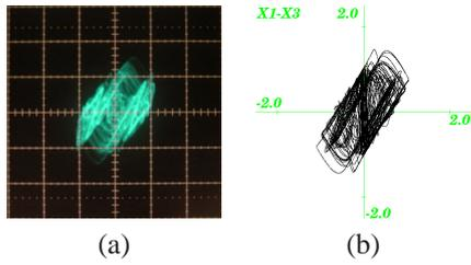
Figure 7: circuit experimental result (a) and computer calculated result (b) of circuit no. 3. (a)horizontal axis:  $v_1$ [0.5v/div], vertical axis: $v_3$ [0.5v/div],  $R_1 = 5.6$ [k $\Omega$ ],  $R_2 = 5.6$ [k $\Omega$ ],  $R_3 = 1.0$ [k $\Omega$ ],  $R_4 = 5.0$ [k $\Omega$ ],  $C_1 = C_2 = C_3 = 33$ [nF],  $L_1 = 50$ [mH]. (b)horizontal axis:  $x_1$ , vertical axis:  $x_3$ ,  $\alpha = 1.0$ ,  $\beta = 4.5$ ,  $\gamma = 1.0$ ,  $\delta = 20$ ,  $\varepsilon = 40$ .
