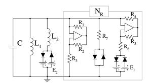
Figure 2: Proposed chaotic circuit with piecewise linear resistors.
