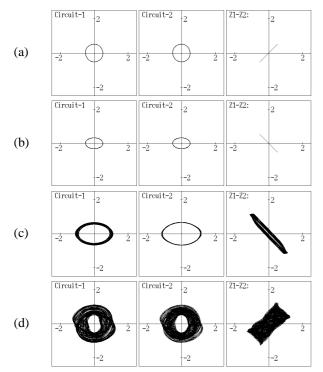
Figure 6: Four oscillation modes exist at the same parameters:  $\alpha = 0.80$ ,  $\beta = 10.0$  and  $\gamma^* = 0.480$ . (a) in-phase synchronous limit cycle, (b) anti-phase synchronous limit cycle, (c) anti-phase chaotic synchronous attractor, (d) double-mode oscillations both of two different attractors chaotic and small size limit cycle.
