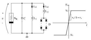
Figure 1: Schematic figure for the chaotic circuit, and a typical characteristic of the diode model with polarities.
