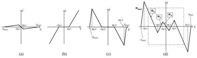
Figure 3: Design method for v-i characteristic of a piecewise linear resistor in the chaotic circuit. Characteristics of (a) N<sub>r1</sub>, (b) diodes and one resistor, (c) N<sub>r2</sub> and ideal diodes with polarities, (d) compound characteristics of N<sub>R</sub> connected by (a) to (c) in parallel.
