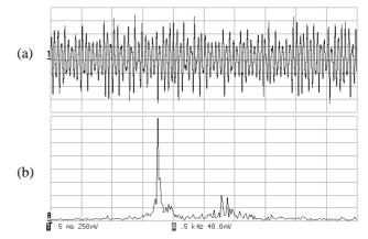
Figure 8: Snapshots of a time waveform and a FFT spectrum at the double-mode chaotic oscillations. (a) time waveform, horizontal: 5[msec/div], vertical: 2.5[V/div], (b) FFT, horizontal: 500[Hz/div], vertical: 400[mV/div].
