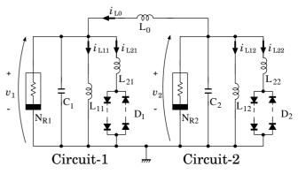
Figure 5: Circuit model of two MSCCs coupled by an inductor.
