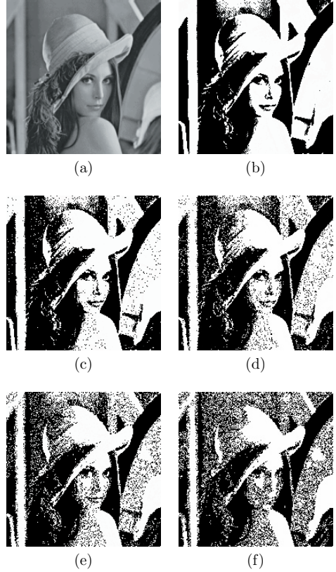
Figure 3: An example for gray-scale image to binary encoding by using SWCNN. (a) is the input and initial state image, (b) is the binary output image for the original CNN. (c)-(d) are the binary output images obtained by using the SWCNN with the probability p = 0.1, 0.3, 0.5 and 1.0, respectively.
