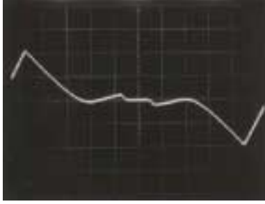
Figure 6: Measured v - i characteristics of the negative resistor.
