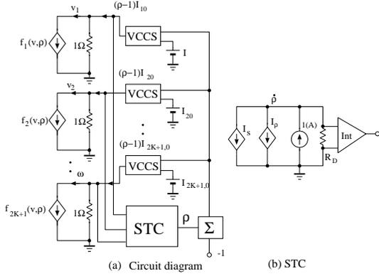
Fig.2 Circuit diagram of the Newton homotopy method
