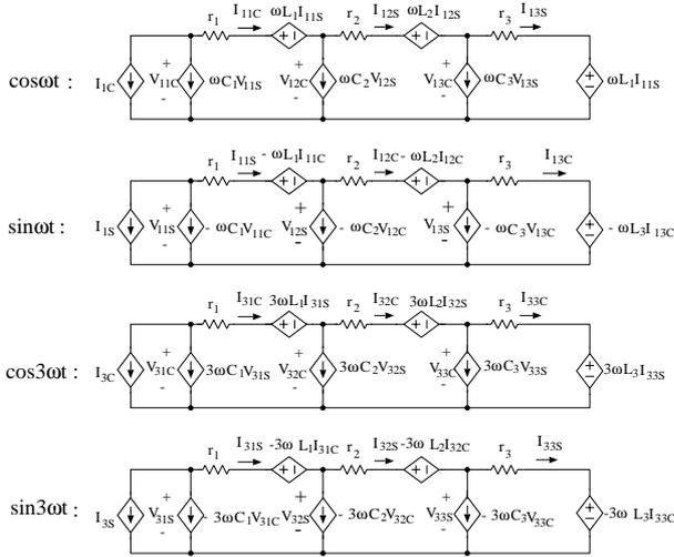
Fig.5 Equivalent circuit describing the determining equation for  $K = 1$
