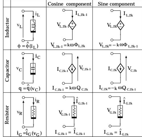
Fig.3 Equivalent cosine and sine circuits
